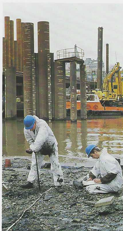
Augering on the Thames foreshore in order to map the buried sediments
