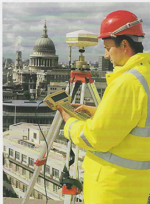
A Leica 200 GPS receiver being used to set up a national grid base line adjacent to the excavations at Number 1 Poultry. GPS allows fast and accurate surveying field work and data processing
