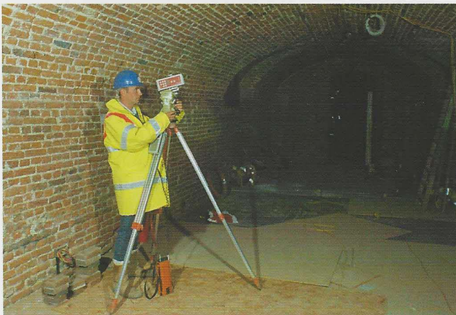
Reflectorless EDM recording of basement vaults of the Queen's House, Greenwich
